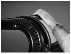
3. Slide the top panel about 1 inch toward the rear of the unit and lift it off.
