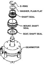
**FIGURE 9. SHAFT SEAL**
