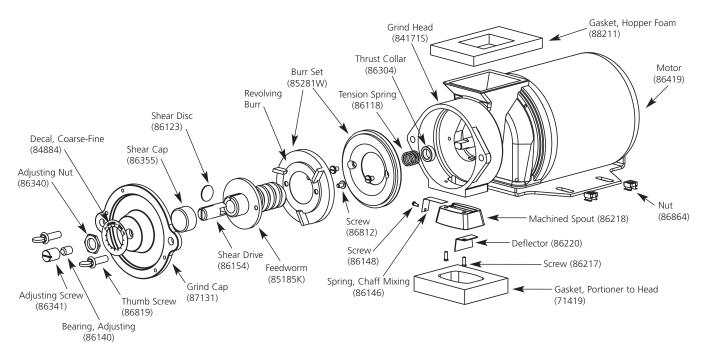
Figure H: Motor Assembly
