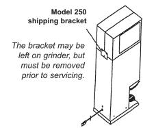
Figure E: Shipping Bracket Removal
