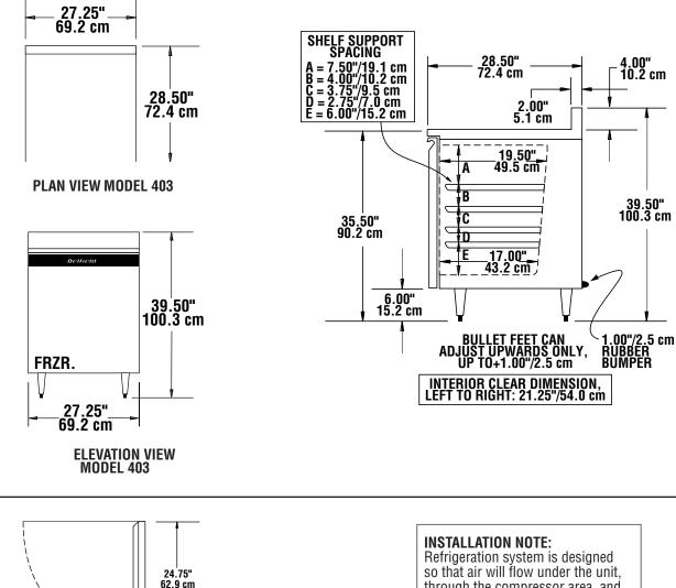
Refrigeration system is designed so that air will flow under the unit, through the compressor area, and out the top rear of the unit. Any restriction to this air flow path will void the warranties.
