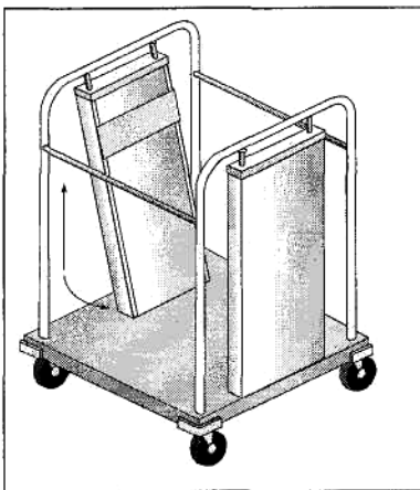
(figure 2) Remove elevator housing
