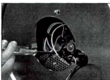
(diagram 3) Location of thermostat adjustment screw
