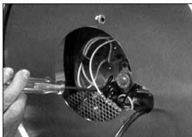
(diagram 3) Location of thermostat adjustment screw
