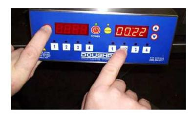
Once you have set the desired time simply press the **TEMP** button, the unit will display the new set-time.
