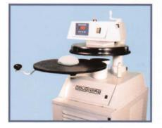
After allowing upper platen to reach desired temperature, swing out lower platen and place pre-portioned ball of dough in approximate center and swing closed. An approved lubricant/release agent such as olive oil or DOUGHPRO's Cookware Food Release Spray # DPPC1 applied to the top of the dough ball will greatly improve the pressing operation.
