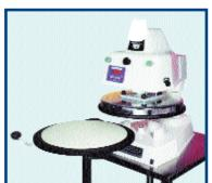
Wait for the automatic pressing cycle to finish. Pull out lower platen and place flattened crust on screen, disc or pan. Now you're ready for make-up and baking.
