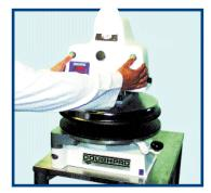
Set the desired time cycle, push down both left and right piston activation buttons, hold until resistance is felt and release. A beeping sound will be heard when it reaches 0.
