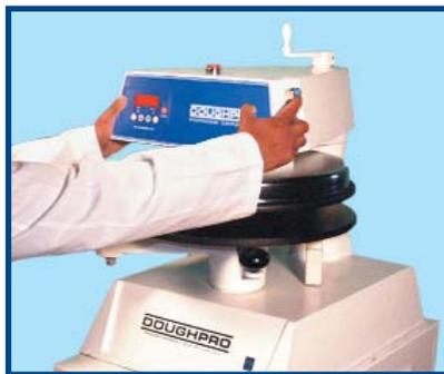
Set the desired time cycle. Push down both left and right compression activation buttons, hold until resistance is felt and release. The DP1300 will automatically release when the time cycle is finished.
