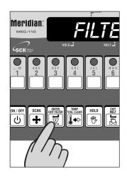
If the controller is programmed for filter lockout, FILTER will appear in the display after the pre-programmed number of cook cycles allowed. The controller will stop operating until the fryer is filtered. After filtering, the display will read FILL. **At this time, the fryer MUST be refilled with oil**. When this step is complete, press ENTER to resume normal operations.
