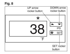
The controller is pre-programmed with a 34 F set point which provides a compressor cut-in at 38 F and cut-out at 34 F. This may not meet your specific application needs. For example, many pharmaceutical manufacturers recommend that their refrigerated medications be stored between 36 F and 46 F. Instructions for changing the set point are found below.
