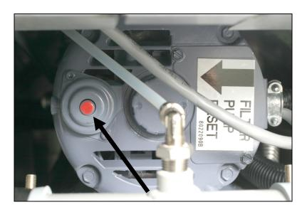
**Filter Pump Reset Switch**
