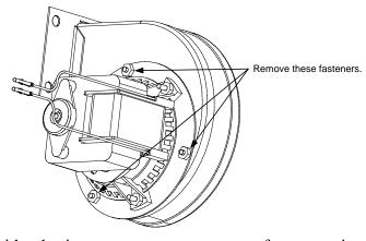
3. Wrap the motor with plastic wrap to prevent water from entering it. Spray degreaser or detergent on the blower wheel and the blower housing. Allow it to soak for five minutes. Rinse the wheel and housing with hot tap water, then dry with a clean cloth.
