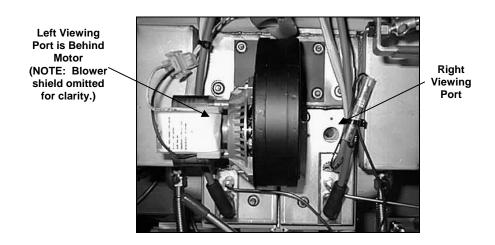
The air/gas mixture is properly adjusted when the burner manifold pressure is in accordance with the applicable table on page 2-7 and the burners display a bright orange-red glow. If a blue flame is observed, or if there are dark spots on a burner face, the air/gas mixture requires adjustment.
