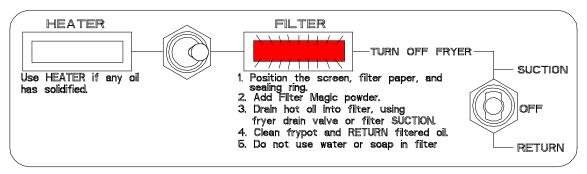
The Heater/Filter switch must be in the FILTER position before the filter pump can be operated. The red light will illuminate when the switch is properly positioned.
