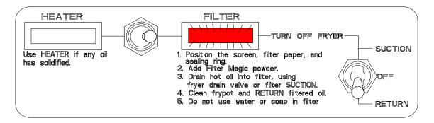
Allow the oil to circulate through the frypot and filter for approximately 5 minutes (process known as "polishing"). Polishing the oil produces maximum filtration and extends the life of the oil. Rinse any residual oil or sediment from the frypot during the polishing process.
