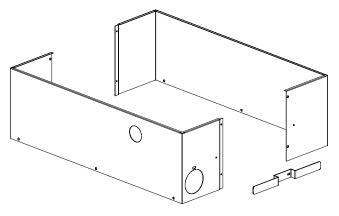
Remove cord-holder bracket and outer panels.
