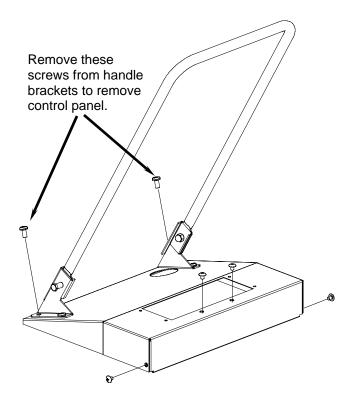
Remove screws illustrated to remove control panel. (Switch panel omitted for clarity.)
