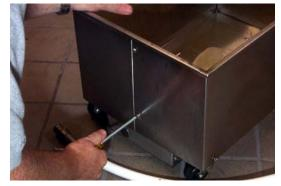
Remove screws securing outer panels.
