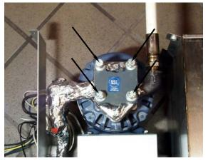
Remove the four bolts securing the pump to the motor (arrows).
