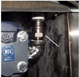
Remove hose fitting (arrow) with an open-end wrench. Use pipe sealant when installing new hose.
