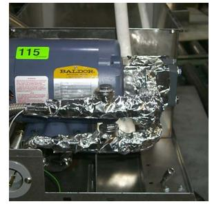
Heater strip installed [115V PF50 (Return/Suction)].
