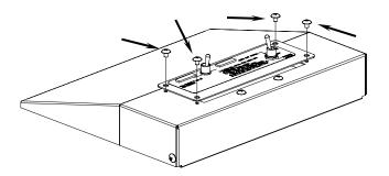
Remove screws (arrows) securing switch panel to the control panel.
