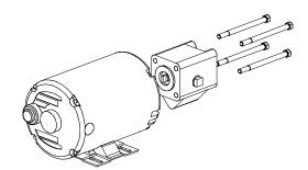
Remove four bolts securing the pump to the motor. Remove pump and gasket from motor.
