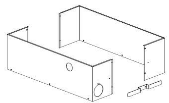
Remove cord-holder bracket and outer panels.
