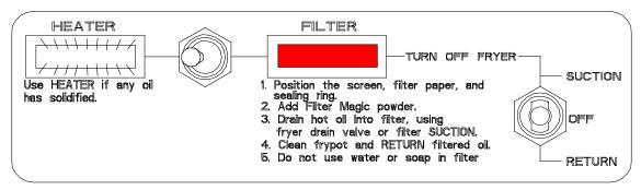
Use the filter heater for 20-30 minutes prior to filtering if solid shortening is filtered.
