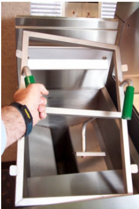
Fig: 12:15 A Power Shower is shown being placed in a frypot. Filtered oil returning to the frypot flows through the device and down the sides of the vessel, cleaning the pot walls.
