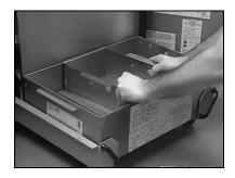
5. Push the filter pan back into the fryer, positioning it all the way to the back of the cabinet. (When the FM II filter assembly is properly positioned, the green HEATER ON indicator will light.)
