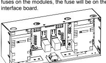
For units in which the ignition module has no fuse, replace the upper fuse on the interface board.
