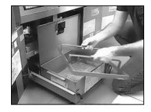
2. Remove used filter paper if present, and clean the pan as necessary. Verify that the metal filter screen is in the bottom of the pan, and then lay a clean sheet of filter paper over the top of the pan, overlapping on all sides.
