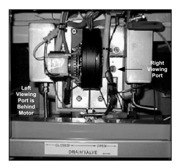
The optimum burn is a bright orange-red glow. If a blue flame is observed, or if there are dark spots on a burner face, the air/gas mix requires adjustment. Adjustment procedures are different for CE and Non-CE units.
