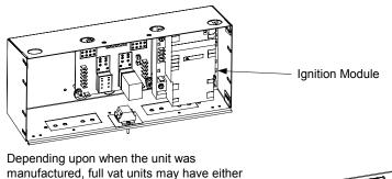
Depending upon when the unit was manufactured, full vat units may have either one or two ignition modules. If there is only one ignition module, the fuse will be mounted on the interface board.
