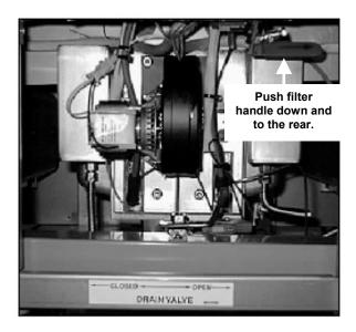
5. After the oil is filtered, close the drain valve and allow the fryer to refill. Let the filter run 10 to 12 seconds after bubbles appear in the oil to clear the lines and prevent hardening of shortening in the lines.
