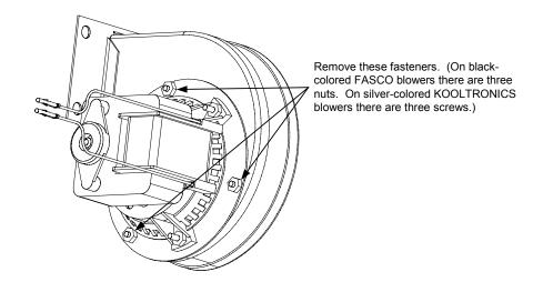
3. Wrap the motor with plastic wrap to prevent water from entering it. Spray degreaser or detergent on the blower wheel and the blower housing. Allow it to soak for five minutes. Rinse the wheel and housing with hot tap water, then dry with a clean cloth.
