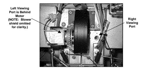
The air/gas mixture is properly adjusted when the burner manifold pressure is in accordance with the applicable table on page 1-7 and the burners display a bright orange-red glow. If a blue flame is observed, or if there are dark spots on a burner face, the air/gas mixture requires adjustment.
