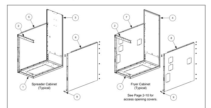
NOTES: Complete Spreader Cabinet Assemblies are: 806-6495SP (S/S) and 806-6496SP (CR). Complete Fryer Cabinet Assemblies are: 806-46232SP (S/S) and 806-46231SP (CR).
