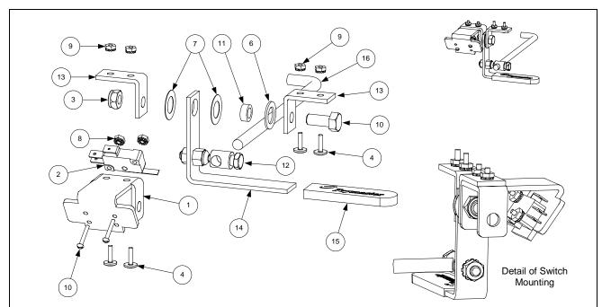
Handle and switch assembly is shown in right-hand configuration (806-3470SP). Left-hand configuration (806-3471SP) is mirror image of 806-3470SP using same components. Oil return valve rod (Item 16) IS NOT a component of either assembly.
