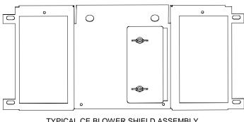
TYPICAL CE BLOWER SHIELD ASSEMBLY ON UNITS BUILT THROUGH APRIL 1999
