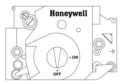
2. Remove the pressure tap plug from the gas valve assembly.
