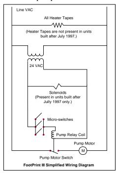
The oil return line heater tapes in the Filter Magic system are wired directly into the line VAC source and remain energized as long as the unit is plugged in. The filter pan suction tube heater tape, however, is wired into the 24 VAC circuit. The suction tube tape is activated only when the filter pan is positioned all the way to the rear of the cabinet, allowing a pair of "bullet" contactors mounted on the pan to touch a corresponding pair of contactors mounted on the cabinet frame.
