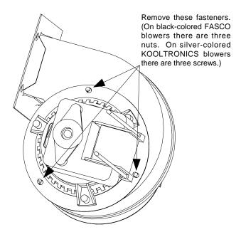
3. Wrap the motor with plastic wrap to prevent water from entering it. Spray degreaser or detergent on the blower wheel and the blower housing. Allow it to soak for five minutes. Rinse the wheel and housing with hot tap water, then dry with a clean cloth.
