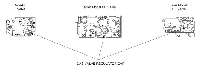
6. Place the fryer power switch (and the gas valve in non-CE fryers) in the OFF position. Remove the fitting from the pressure tap hole and reinstall the pressure tap plug.
