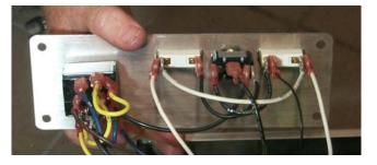
Mark wiring locations on defective switch/light before disconnecting wires.
