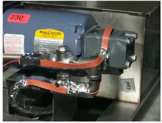
Heater strip routing on flexlines and pump [230V PF50 (Return/Suction)].
