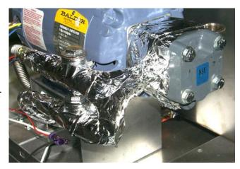
Remove foil insulation tape covering the heater strip and remove heater strip from the pump and flexlines. Disconnect the flexlines from the check valve connections.
