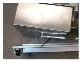
Remove foil-insulating tape to expose heater strip (arrow).
