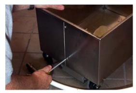
Remove screws securing outer panels.
