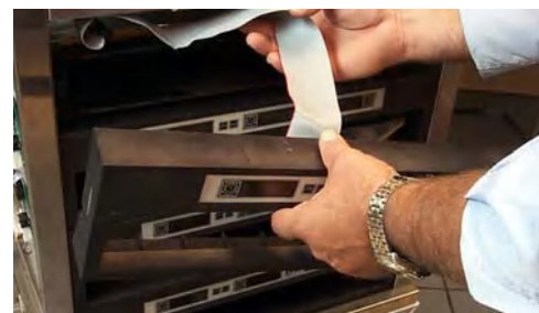
Fig. 7. Feed ribbon cable out of UHC when bezel is removed.
