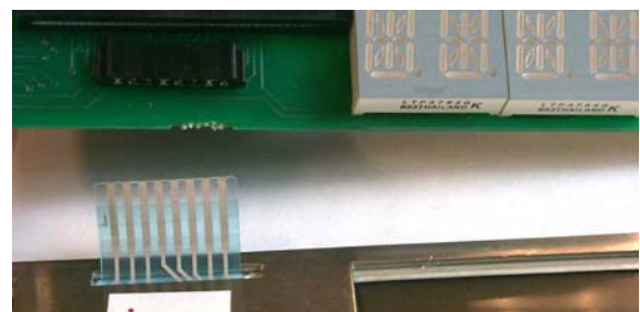
Fig. 11. The ribbon on the membrane switch is pulled free of the connector on the display board.
