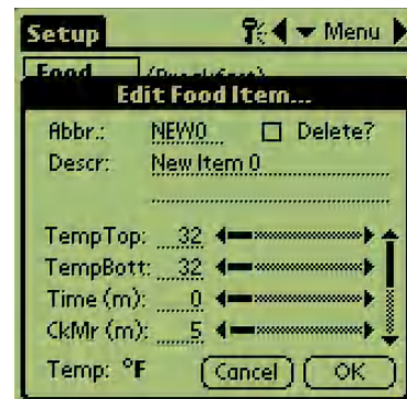
Step 3: The Edit Food Item menu appears. It allows the product to be named and holding temperatures, times and Cook More prompts to be entered.
