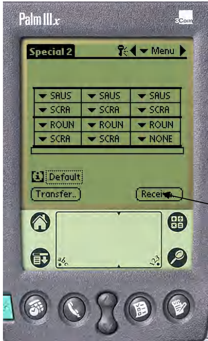
Figure 1: To prepare the Palm Pilot to receive data from the UHC-P cabinet, tap the receive button.
