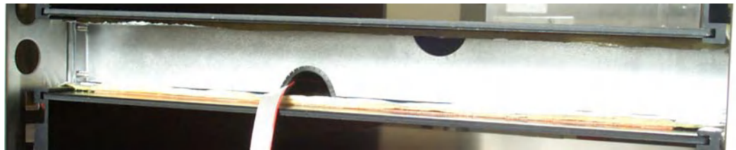
Figure 10: A baffle is secured behind the bezel.
