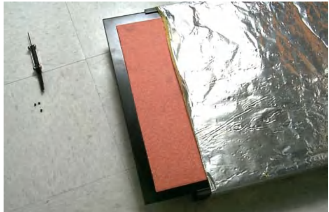
Figure 9: The heater plate slides from the insulation.
