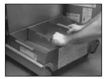
7. Push the filter back into the cabinet, making sure that it is positioned all the way to the back. (When the FM II filter is properly positioned, the green HEATER ON indicator will light.)
