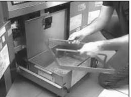
2. After verifying that the metal filter screen is in the bottom of the pan, lay a sheet of filter paper over the top of the pan, overlapping on all sides.
