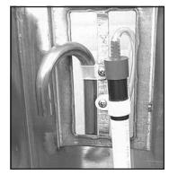
Stainless Water Inlet Tube and Low-Level Sensor Pick-Up Tube (Cover Removed)
