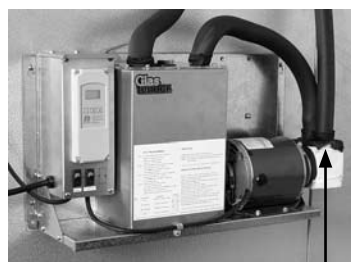
Connect glycol recirculating line from pump outlet 3/8" barb fitting to the beer line set.
