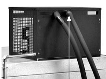
Connect glycol recirculating line from beer line set to the return 3/8" barb fitting.
