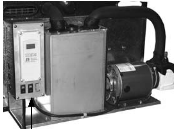
Remove control cover to get at the power cord. Disconnect 33" power cord.
