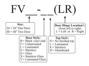
† The door on the FV24 may hinge either Left or Right. The hinges on the FV48 are only available as LR.
