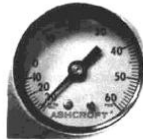
Correct vacuum reading for cold kettle
