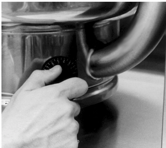
A simple turn of the thermostat controls the Groen TDB/6 Kettle.
