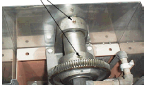
Add grease through Zerk Fittings.
