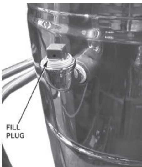
To add water to the jacket, , remove the fill plug. (Note the venting holes)
