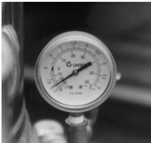
The pressure gauge should show a vacuum of 20 to 30 inches when the kettle is cold.
