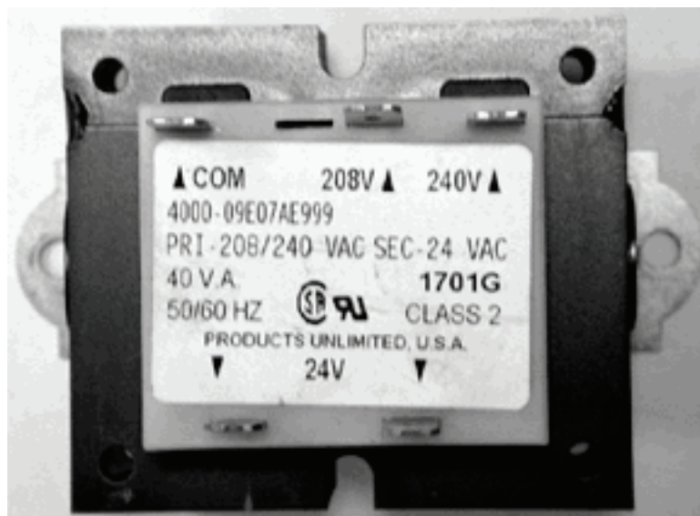
Photo #1 Pull lead from 208V tab and insert on 240V tab.
