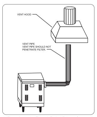
Figure 8. Venting Through Typical Exhaust System.
