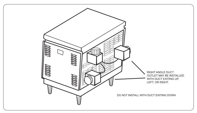
Figure 10. Right Angle Adapter Mounting Options.
