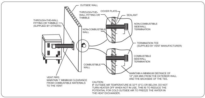
Figure 9. Typical Through-the-Wall Venting
