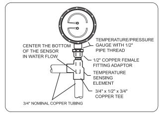
Figure 2. Installation Temperature/Pressure Gauge
