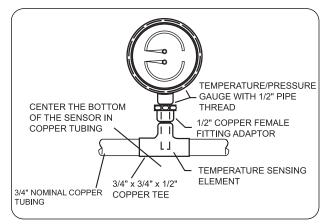
Figure 3. Installation Temperature/Pressure Gauge
