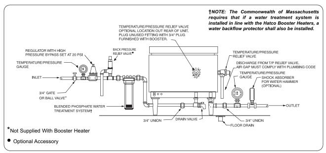
Figure 4. Plumbing Connections – PMG-100/200 Gas Booster Heaters
