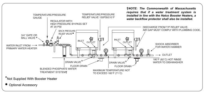
Figure 5. PMG-100/200 Gas Booster Heaters Connected in Series
