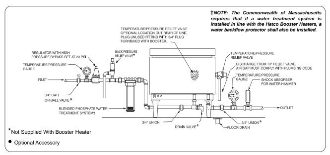
Figure 4. Plumbing Connections – PMG-60 Gas Booster Heater
