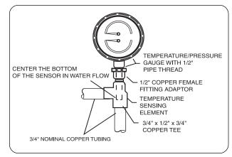
Figure 2. Installation Temperature/Pressure Gauge
