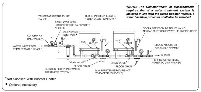
Figure 5. PMG-60 Gas Booster Heaters Connected in Series
