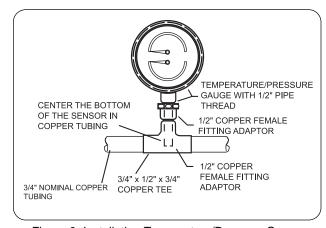
Figure 3. Installation Temperature/Pressure Gauge
