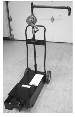
10. Replace and latch the cover and roll oil disposal shuttle to disposal container.
