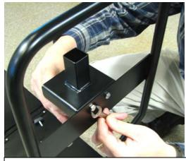
BOLT BRACKET TO HANDLE WITH BOLTS PROVIDED AND SLIDE PUMP AND TUBE ASSEMBLY THROUGH SQUARE TUBE AND INTO ROUND TUBE.
