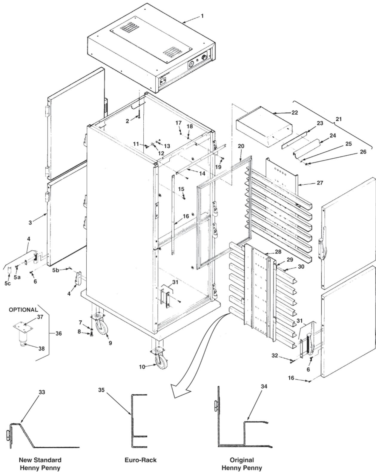
Figure 3-2. Cabinet Assembly - UL & CE Approved
