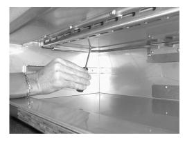
4. Using a Phillips head screwdriver, remove the ten screws securing the bracket and remove the bracket.
