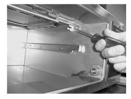
3. Using a flat blade screwdriver, pry the rubber strain relief from the liner.
