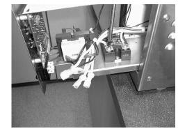
8. Using a Phillips head screwdriver, remove the screws securing the relay and remove the relay from the unit.
