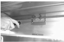
5. Using a Phillips head screwdriver, remove the two screws securing the element to the back of the liner.
