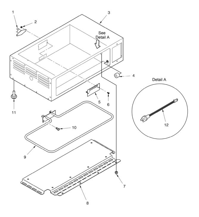
Figure 2-2. Heater and High Limit
