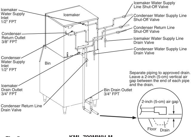
Fig. 5 KML-700MWH-M Connection to a Closed Loop System
