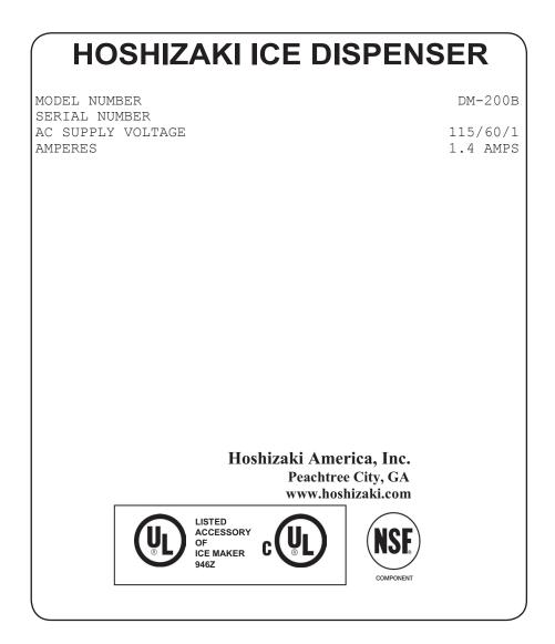
See the nameplate for electrical specifications. This nameplate is located on the upper right hand side of the rear panel.
