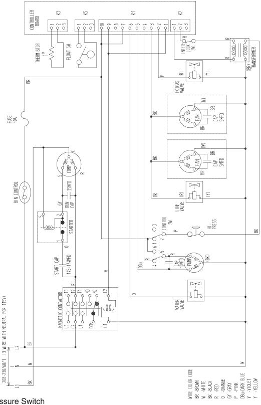
Note: Pressure Switch Cut-out  $412_0^{+21.3}$  PSIG Cut-in 327  $\pm$  21.3 PSIG
