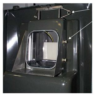
Begin by removing the sink assembly. Check the action of the ice chute and return springs.
