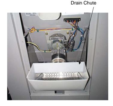
Pull out the drain chute. Clean out any debris that might be in the chute or screens.
