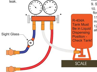
Hose Connection Schematic for Liquid Charging
