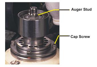
•unscrewing the auger stud
