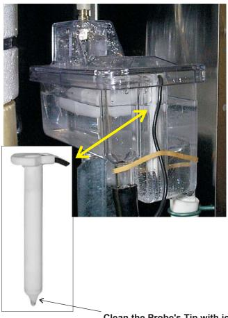
Clean the Probe's Tip with ice machine cleaner and a clean, soft cloth.
