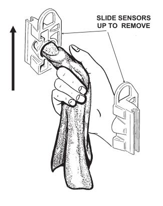
2. The bin control uses devices that sense light, therefore they must be kept clean enough so that they can "see". At least twice a year, remove the bin control sensors from the ice chute, and wipe them clean.
