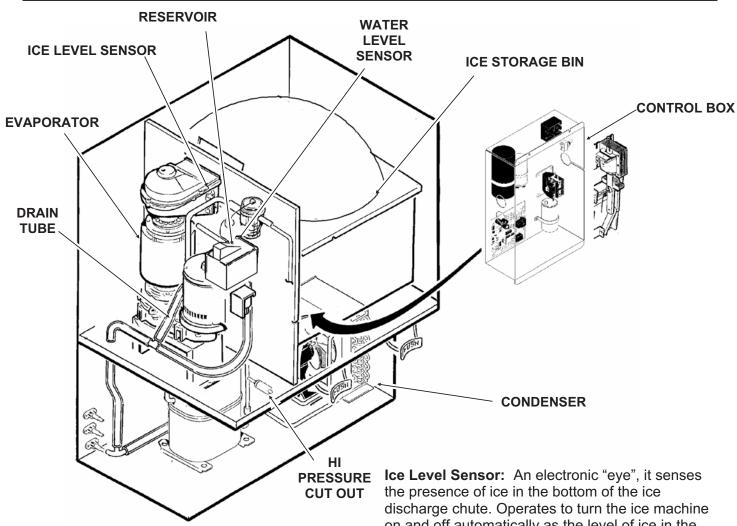
Control Box: Contains the electrical controls that operate the machine.
