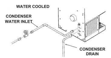
Water Cooled Models: In addition to the above mentioned drain, a separate condenser drain line must be installed. Connect it to the  $\frac{1}{2}$  " condenser drain connection at the back of the cabinet.
