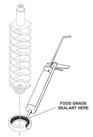
2. Replace the snap ring and pull the water seal down against it.
