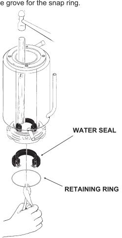
5. Carefully push the water seal (rubber side against the auger shoulder and the silastic sealant.)
