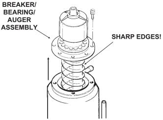
a. Unscrew 4 allen head cap screws holding breaker to evaporator.
