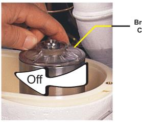
Breaker Cover • unscrewing the breaker cover.
