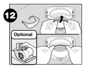
Place a weight such as the disposer on the sink flange to hold it in place. Use a towel to prevent scratching sink. Pull snap ring open and press firmly until it snaps into place.
