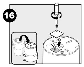
Turn disposer over and remove electrical cover plate.
