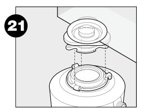
Hang disposer by aligning 3 mounting tabs with slide-up ramps on mounting ring.
