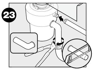
You may need to trim tube for proper fit. Reconnect plumbing (and dishwasher or direct water connection if used). Make sure tailpipe mount is straight.
