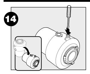
Turn disposer onto side and insert screwdriver into dishwasher inlet.
