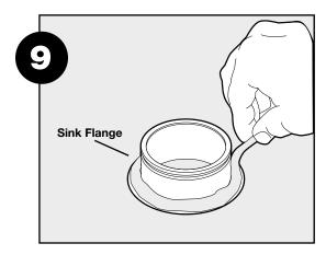
Evenly apply 1/2" thick rope of plumber's putty around new flange.
