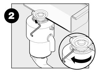
Support disposer, insert end of wrenchette into right side of mounting lug, and turn. Disposer will fall free.
