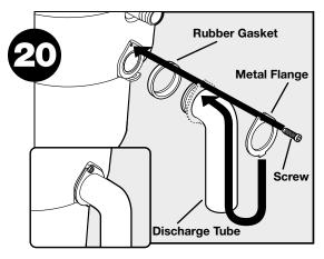
Rotate the disposer around. Place the rubber gasket on the end of the discharge tube and slide on the metal flange from the reverse end. Place assembled discharge tube in the tailpipe mount opening and secure with screw provided.
