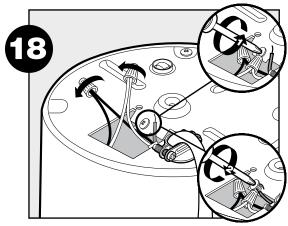
Connect white to white and black to black or red with wire nuts (not included); ground wire to green grounding screw. Unit must be grounded for safe and proper installation.
