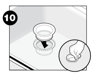
Press flange firmly into sink drain. Remove excess putty.
