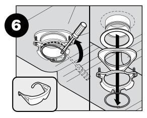
Using a screwdriver, remove the snap ring.
