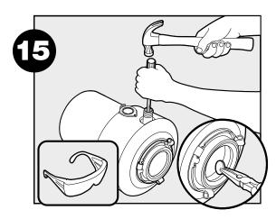
Knock out drain plug and remove plug from inside of disposer.
