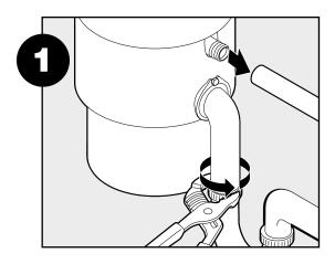
Disconnect drain trap from waste discharge tube. Disconnect dishwasher or direct water connection if connected to the disposer.
