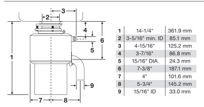
NOTE: Plumb 1-1/2" (38.1 mm) waste line to prevent standing water in disposer motor housing.
