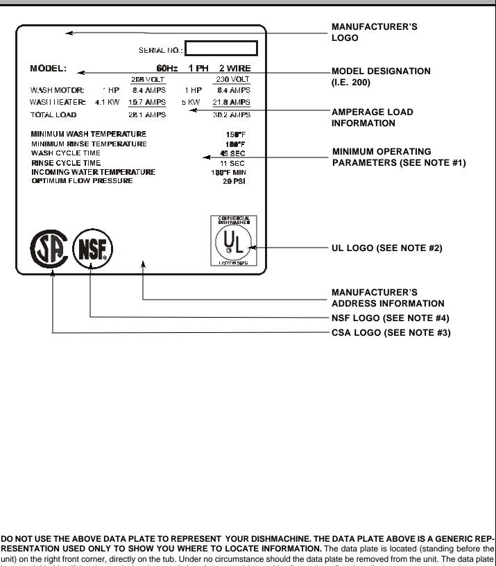
unit) on the right front corner, directly on the tub. Under no circumstance should the data plate be removed from the unit. The data plate is essential in identifying the particular characteristics of your machine and is of great benefit to installers, operators, and maintenance personnel. It is recommended that you copy down the essential information on the final page in this manual for reference before installation.
