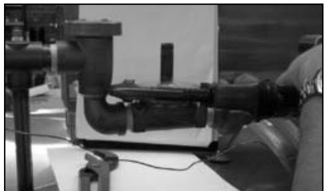
Loosening the valve bonnet
