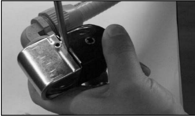
Prying open the coil wire cover
