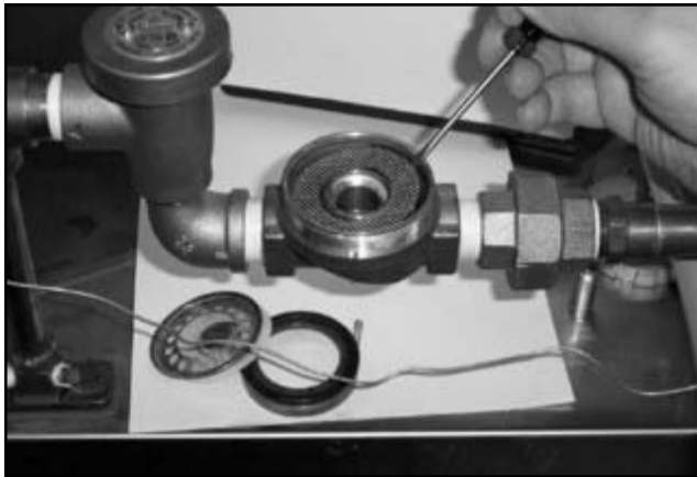
Removing the mesh strainer screen
