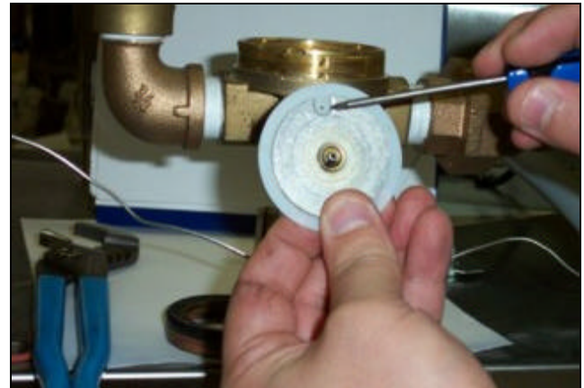
Pointing out the extension hole
