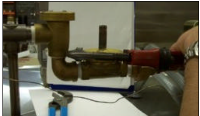
Loosening the valve bonnet
