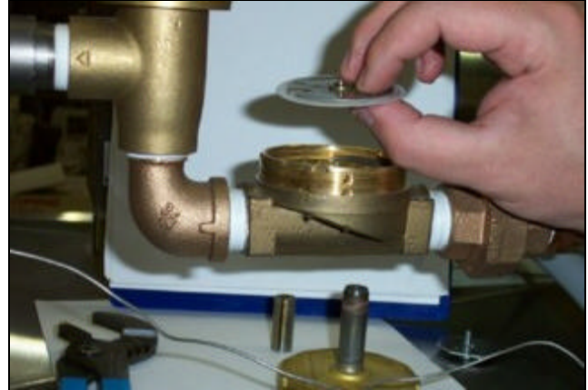
Removing the diaphragm
