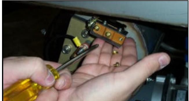
Removing the thermostat screws.
