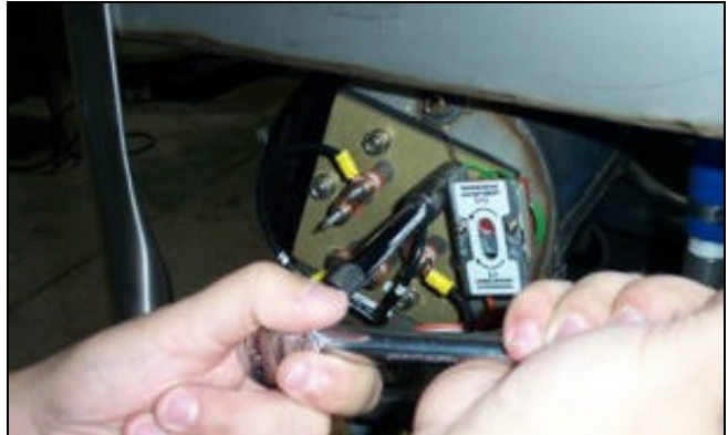
Removing the thermostat bracket/heater nuts.
