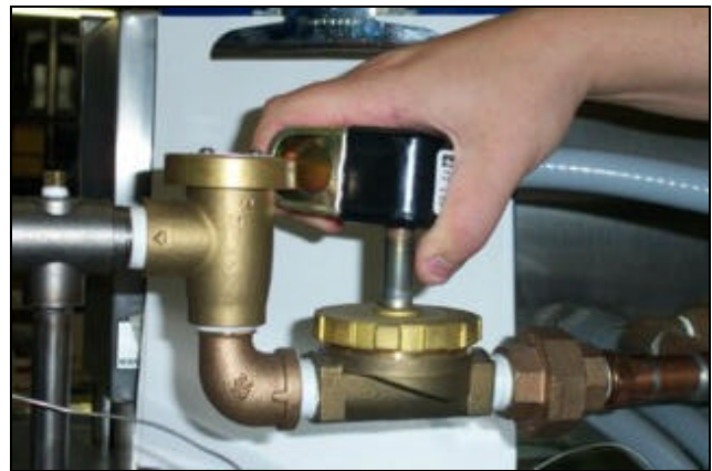
Removing the coil
