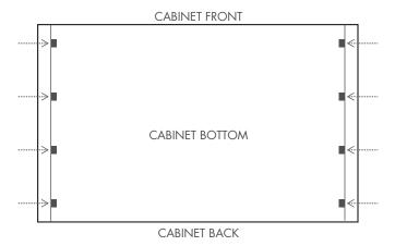
2. Place new leg channels in the small holes against the cabinet side. Return the Hex Screws to their original holes, starting with the center two screws.
