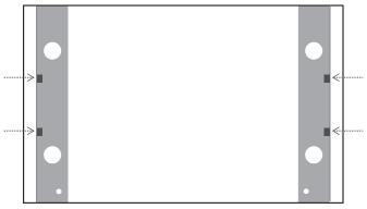
**3.** Tighten your screws with the <sup>3</sup>/<sub>8</sub>" Socket Wrench on an extension through the leg channel.
