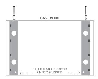
of the cabinet bottom and leg channel. The holes for this exist and will be inline if the leg channel is installed properly. Secure with 1/4"-20 Serrated Flange Nut (part # 031567).
