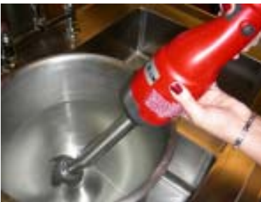
1. Immediately after use, place 2/3 of the mixer arm into hot water and switch on for a few seconds.
