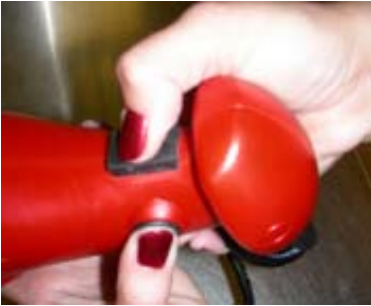
4. Press Start button and Safety button at the same time. Releasing the Start button will cause the machine to stop operating.
