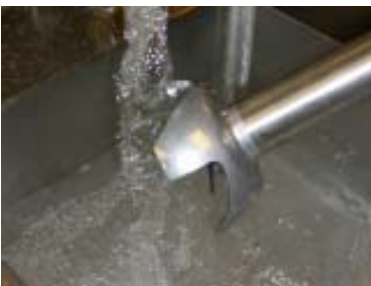
4. Rinse the mixer arm and blade with warm water to remove any residue.
