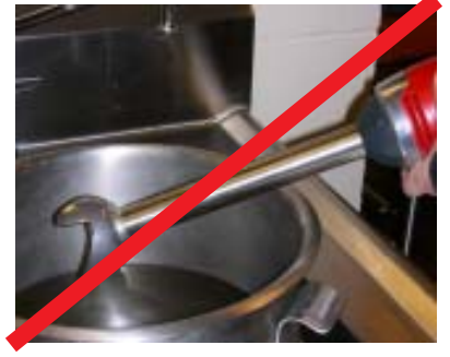
3. To prevent food getting inside the motor, DO NOT incline machine more than 30°.
