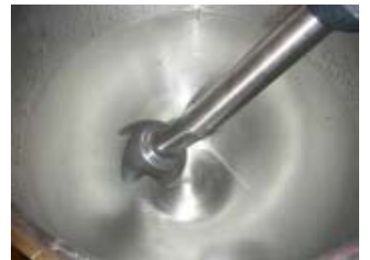
3. The mixer blade must be cleaned with hot water and mild detergent, leaving the blade submerged for 30 minutes.
