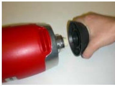
2. To remove mixer arm, turn the mixer clockwise until the arm separates from the motor set.
