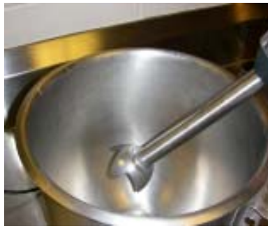
2. Insert arm of machine into bowl, up to 2/3 of the mixer arm's length. Do not let the foot of the machine touch the bottom of the bowl.
