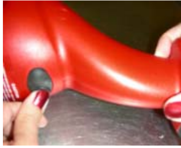
5. While the machine is running, press the Lock button. After the Lock button is depressed, the Start button may be released and the machine will continue to operate.
