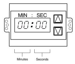
Figure 3-3. Conveyor Speed Digital Control
