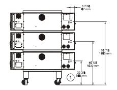
Figure 2-7. MODEL PS536ES TRIPLE OVEN DIMENSIONS
