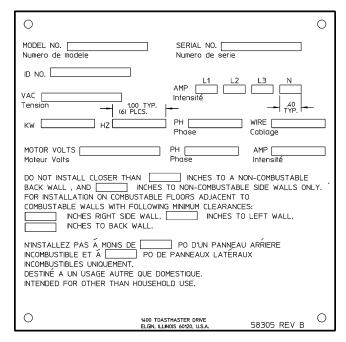
Figure 2-11. Typical Electric Oven Data Plate
