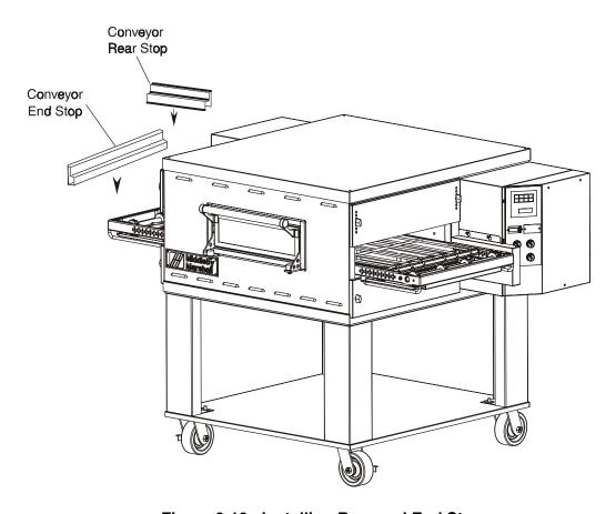
Figure 2-13. Installing Rear and End Stops
