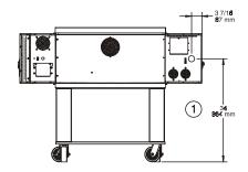
Figure 2-6. MODEL PS536ES DOUBLE OVEN DIMENSIONS
