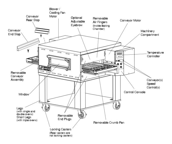
Figure 1-6. PS536ES-Series Oven Components Locations
