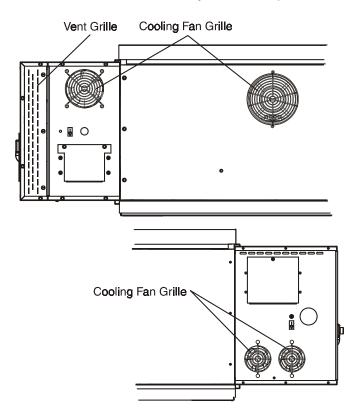
Figure 4-1. Oven Cooling Fans
