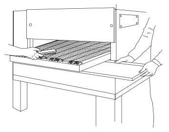
Figure 4-2. Conveyor Belt and Crumb Pan Cleaning
