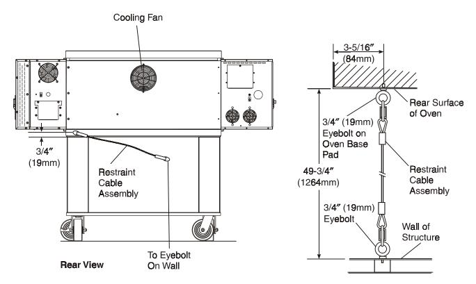
Figure 2-8. Restraint Cable Assembly Installation
